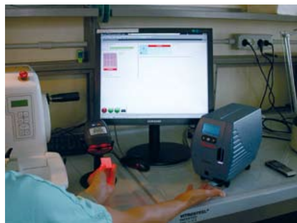
Fig. 5. Cutting station: the cassette is read by the scanner, the LIS shows all tissue block information (patient name and surname, code number, tissue type, number of fragments, embedded status, operator and date) and the slide Mate printer prints the relevant information on the slide.
