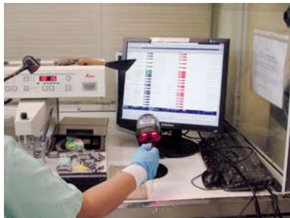
Fig. 4. Tissue embedding station: the cassette is read by the scanner. The LIS displays all relevant information and shows a list of embedded cassettes.
